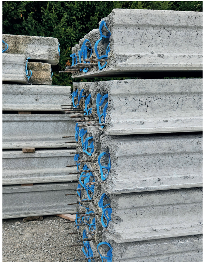
Hollowcore slabs with exposed pre-stressing wires
