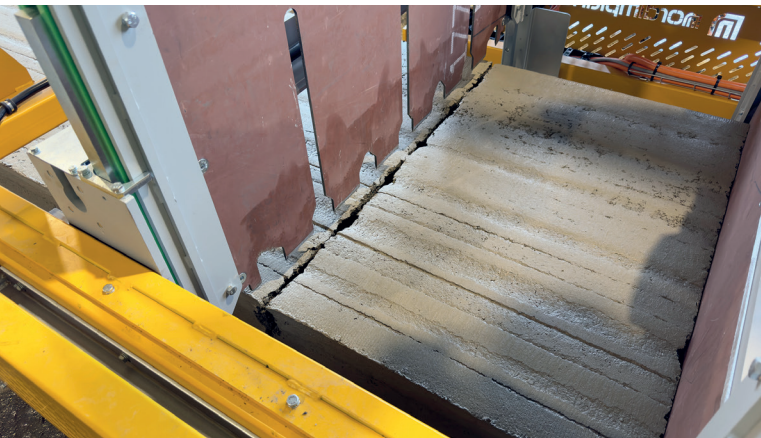
Fresh concrete guillotine cutting assembly
